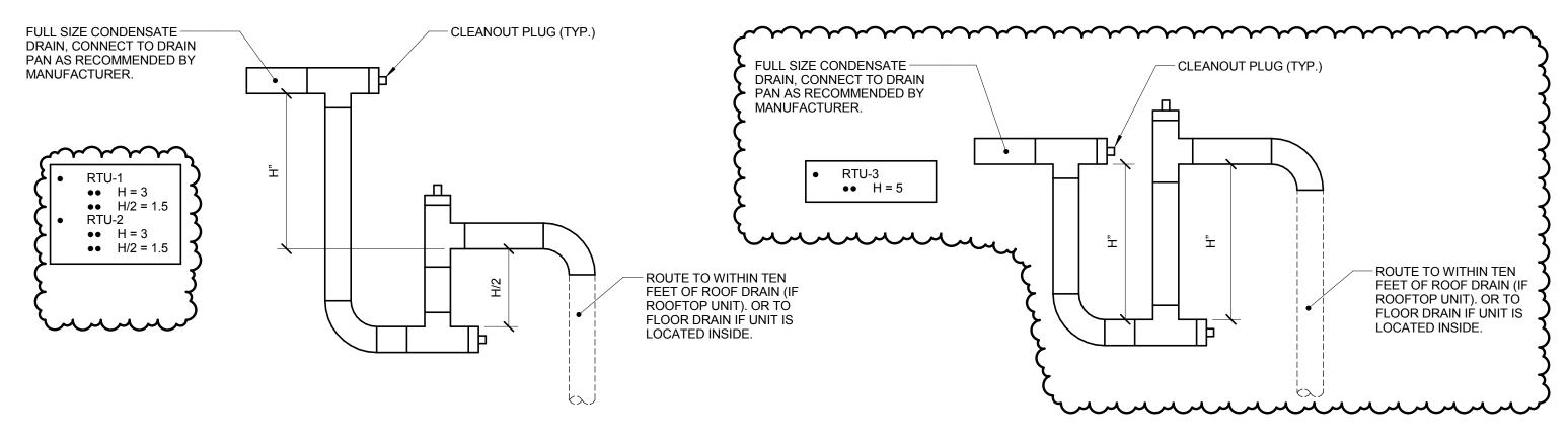
**CONDENSATE TRAP DETAIL** (DRAW-THROUGH) NO SCALE
